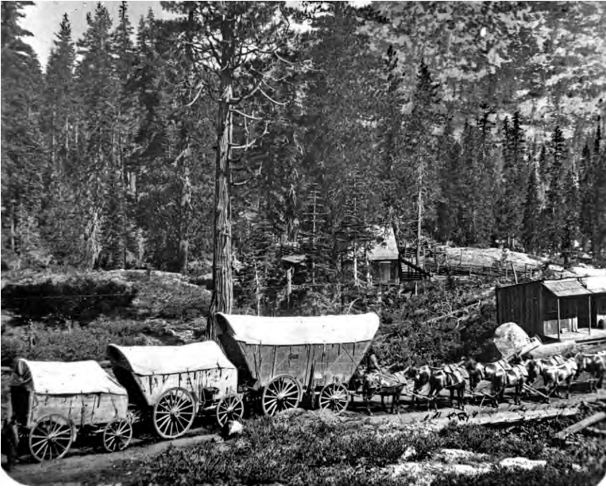
Figure 15 Freight wagons on the road headed to Tahoe and Northern Nevada mining region. The lead wagon shown here is called a Washoe Wagon because of its use to deliver large loads of supplies to the Washoe mining region in Northern Nevada. (Library of Congress Public Domain)
