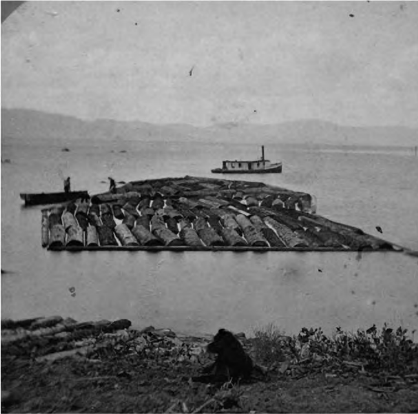
Figure 26 Boom of logs prepared for towing across the lake to the sawmill (University of Nevada Special Collections)
